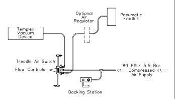
Note: Use of a filter regulator is not necessary when using a Templex Lite Touch Treadle Rod Air Switch with built in flow controls
