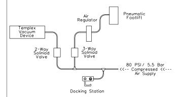
Note: A 3-way solenoid is necessary to operate a single acting air cylinder Proper pneumatic connections using a Templex Lite Touch Treadle Rod Air Switch.
